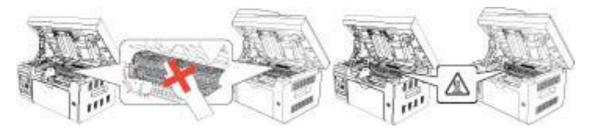
Note: • When removing the laser toner cartridge, put the cartridge in a protective bag or wrap it with thick paper to avoid direct light damaging the photosensitive drum.
