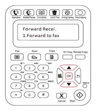
4) When the input is complete, press the OK button and the received Fax will be automatically forwarded to the specified Fax number.
