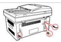
2. Use a soft cloth to wipe the outside of the printer and remove the dust .
