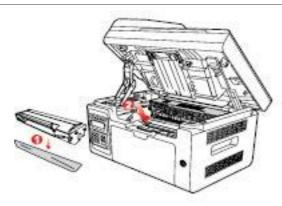
Note: • Check whether there is any seal before installing the laser toner cartridge into the printer; if there is any, please tear off the seal and then install the cartridge.
