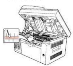
8. Clean the inside of the printer by using a dry and lint-free cloth to gently wipe the shaded area as shown in the picture below.
