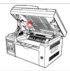
2) Open the output bin by the upper right ridge of the concave section.
