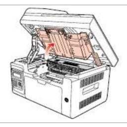
3) Remove the laser toner cartridge along the guides.
