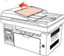
2) Load the manuscript into the automatic document feeder with the front-side up and the top of the manuscript entering into the feeder first.
