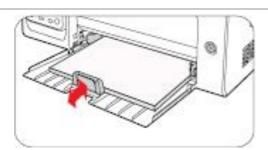
Note:• If the paper loaded into the automatic feeder tray at one time exceeds 150 pages, paper will jam or cannot be fed in.
