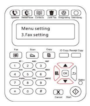
2) Press the OK button to enter the Fax setting options and press the up button "▲" or the down button "▼" to enter the Fax settings.
