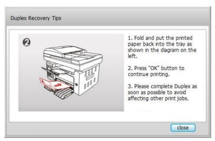
f) After turning over the paper according to the prompt, press "OK" button of the printer to go on printing the other side.
