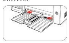
c) Raise the output tray to avoid the paper from slipping and falling.
