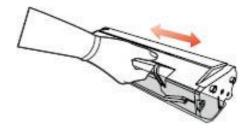
5. Remove the cartridge protector (blister cover), insert the cartridge along the guides into the printer, then push it firmly along the direction of the arrow until you hear a "click" assuring you that the cartridge is fully inserted.
