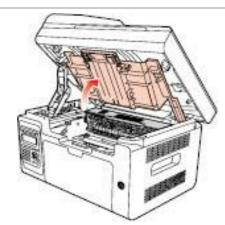
3. Remove the exhausted cartridge along the guides.
