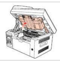
6. Remove the laser toner cartridge along the guides.
