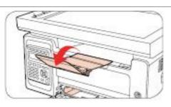
d) Load the paper into the automatic feeder tray with the print-side up.
