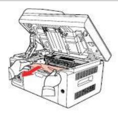
5) After removing the jammed paper, insert the laser toner cartridge into the printer along the guides until you hear a "click" assuring you that the cartridge is fully inserted.
