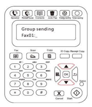
4) When the input is complete, press the Start button to start scanning documents.
