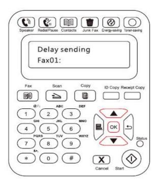
4) When the input is complete, press the OK button to scan the Fax document to the memory and get back to Ready state.
