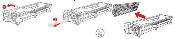
6. Install the drum component along the inner track to finish installing toner cartridge.
