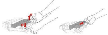
4. Open the package of the new toner cartridge and hold the toner cartridge handle to shake it left and right for 5-6 times, so that the toner inside can be uniformly dispersed.
