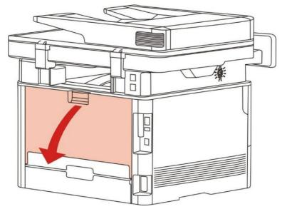
3. Open the fuser door using the handles on both sides.
