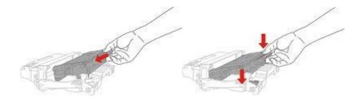
6. Take the drum component with toner cartridge installed and install it inside the printer along the inner track of printer to finish installing.
