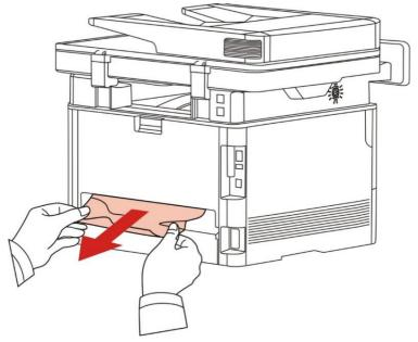
4. After taking papers jammed out, install the duplex unit back and inspect other parts to the product. If it can be ensured that there are no jammed papers, open and close the front cover and then the printer will recover printing automatically.
