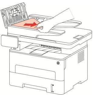
3. After removing the paper jamed, close the top cover and then the printer will be back to the ready state.
