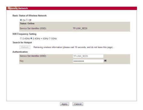
2. If you need to configure a wireless network, turn on the basic status of wireless network, and then click the SSID of the access point (wireless router) in the search list of hotspots, enter the secret key in the authentication, and click Apply.
