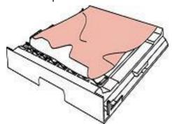
3. If the paper does not come out along with the duplex unit, open the tray and remove the jammed paper directly from the bottom.
