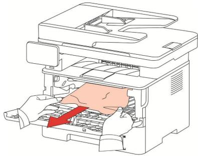
7. After taking out papers jammed, install the laser toner cartridge again and close the front cover, then the printer will recover printing.
