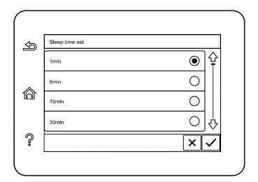
Note: In sleep mode, the printer can be woken up by pressing any key or sending printing work.
