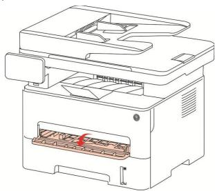
3. Slide the paper deflector of manual feed tray to match the two sides of paper. Do not use excessive force; otherwise, paper will be made jammed or skewed.
