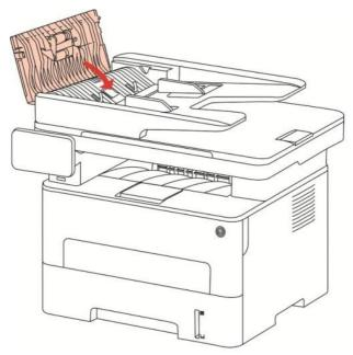
4. If it is difficult to remove the paper jammed, please try to open the scanner cover and remove it from the pressing block.
