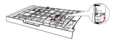
4. Install the duplex unit in the printer.
