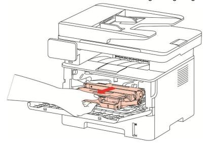
3. Press the blue button on the left side of drum component with left hand and lift the toner cartridge handle with right hand at the same time to take the toner cartridge out.
