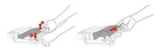
4. Open the package of new drum component, take the protection device of drum component, and put the drum component on a horizontal table.
