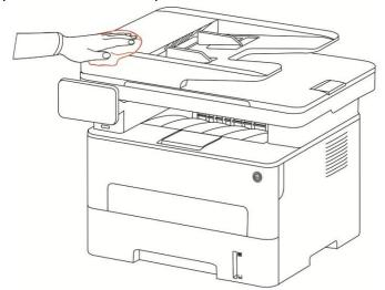
2. Lift the scanner cover, and gently wipe the glass platen and automatic duplex document feeder CIS (D-CIS) with soft cloth.
