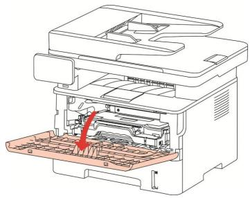
5. Take the laser toner cartridge out along the track. (For the purpose of preventing printing quality from affecting by the exposure of photosensitive drum, please put the laser toner cartridge inside the protection bag or warp it with thick paper).
